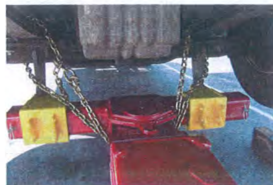
↑ A motorhome built on a truck chassis with standard axles can be towed safely by lifting the I-beam axle, as shown here, and adding chains to secure the lift to the axle.
